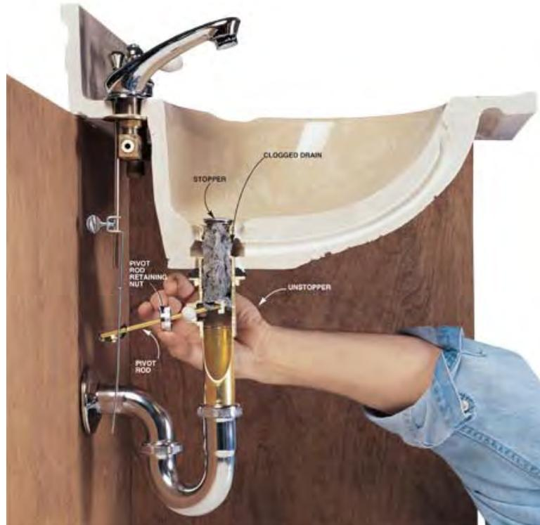
The most common problem with kitchen sinks is the buildup of grease and food particles in the “p-trap” or foreign objects getting stuck somewhere in the drain.
